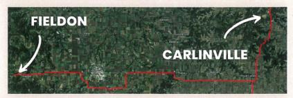
The project pulls ground water from the IL River Bottom near Fieldon, filters the raw water through a water treatment plant, and then conveys the potable water to Carlinville. Clean drinking water hits all the member communities along the way.
